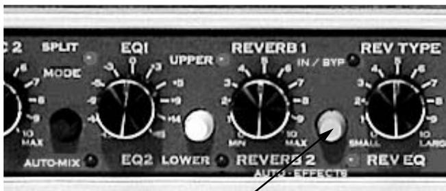
Pressing in and Holding the Reverb IN/BYP switch allows you to Manually Edit in the Auto-Edit Mode if you do not wish to Sing when you use the Editing Function.
